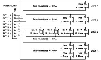
diagram 4 Connection of low-impedance loudspeaker systems
